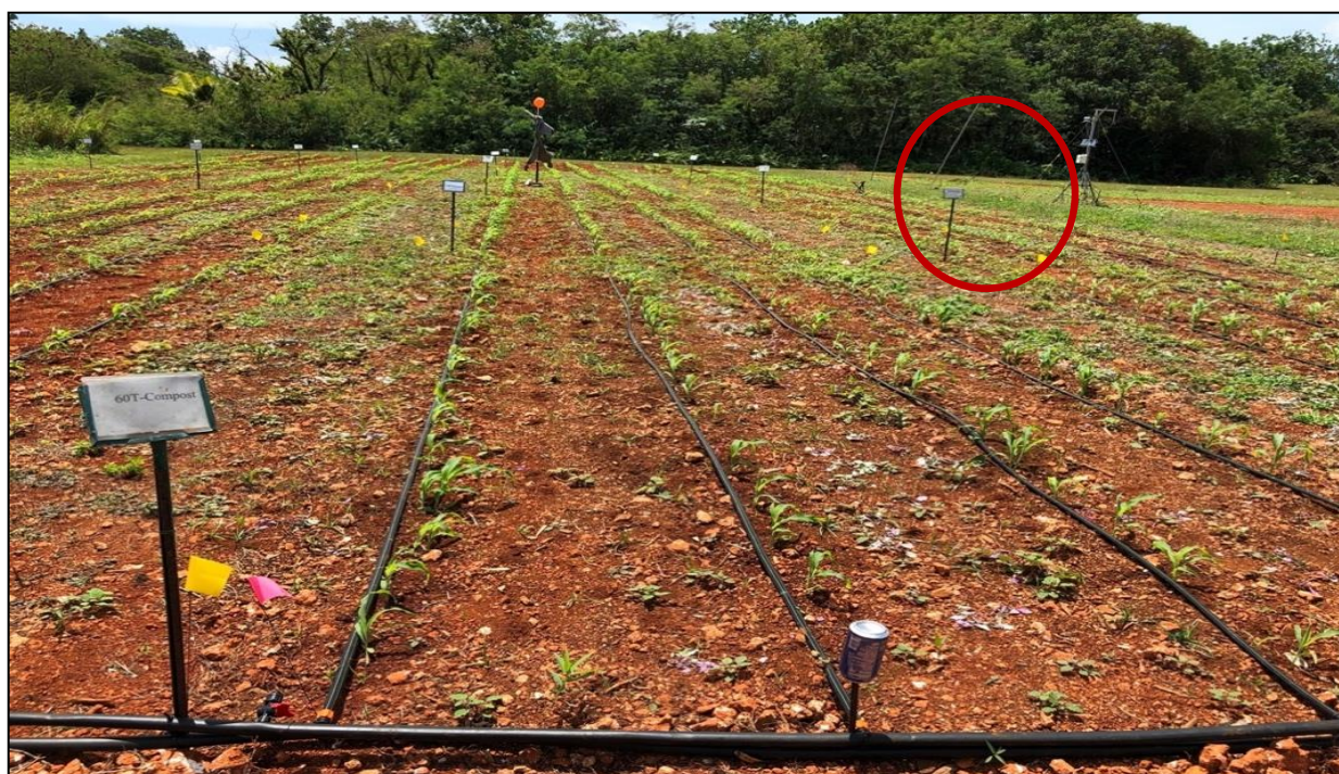
Figure 4: A Weather Station Data Logger (Red Circle) Was Used for Efficient Irrigation.
