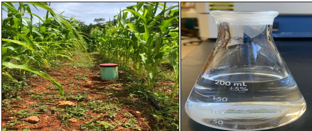
Figure 3: Sealed Containers With 3M Of Sodium Hydroxide-Filled (NaOH) Erlenmeyer Flasks Were Placed Above the Soil Surface to Capture CO 2 Efflux In 24 Hours.
