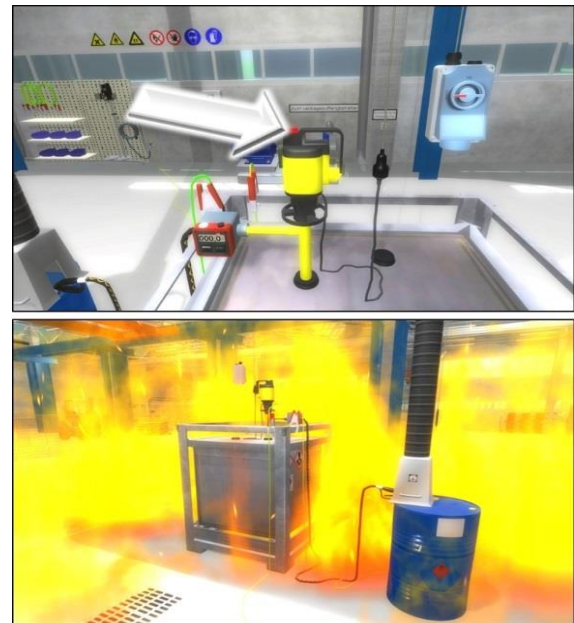
Figure 3: Activation of an inappropriate pump.
